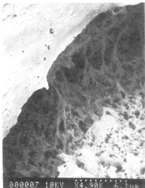
Figure 15. Scanning electron micrograph of the cross-section of a PMMA membrane. The membranes were prepared by quenching a 5 wt % PMMA solution to 27 °C and holding for 5 min. The dense surface is the surface in contact with the thin aluminum sheet.
